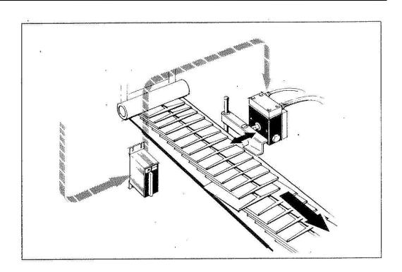
At the discharge on a carton-folding machine, the folded cartons are fed to a distribution conveyor. Subsequent carton handling can be made easier by grouping the conveyed cartons. This is achieved by displacement of a carton at pre-determined intervals.
